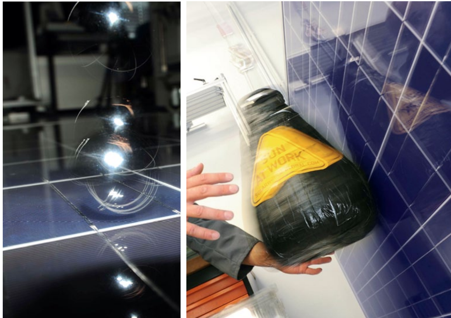
☀ From left to right: Hail impact test | Module breakage test
